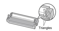
Tap on the toner cartridge several times to allow the toner to fall into the drum unit. Grab the tabs, and shake the drum and toner unit horizontally several times.
